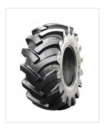
The Primex LS Xtreme features a variable angle lug design that is tapered from the center to the shoulder. This delivers excellent hillside stability, superior traction and exceptional performance in varied ground conditions. The LS Xtreme is engineered with a highly cut and chip resistant compound as well as heavy sidewall and undertread gages for added protection in demanding service.
