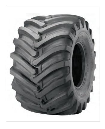
The Primex Terra Turbo II uses a unique dual angle tread pattern. With a 45 degree angle in the center for increased traction and roadability and a 15 degree angle at the shoulder for better turning in the field and less soil disturbance. This tire is designed for maximum performance for drive wheel and free wheel applications.
