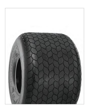
This tire has the weight distributed across a huge footprint for less compaction and turf disturbance. It's shallow tread depth and wide width are for high flotation purposes. Its design allows low inflation pressures to provide flotation over loose soil and sand.
